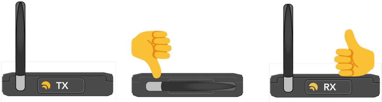
Fig.1: It's important that all antennas point to the same axis – wireless waves have a radial pattern that should be valued. There are a number of accessories that can help maintaining directionality.
